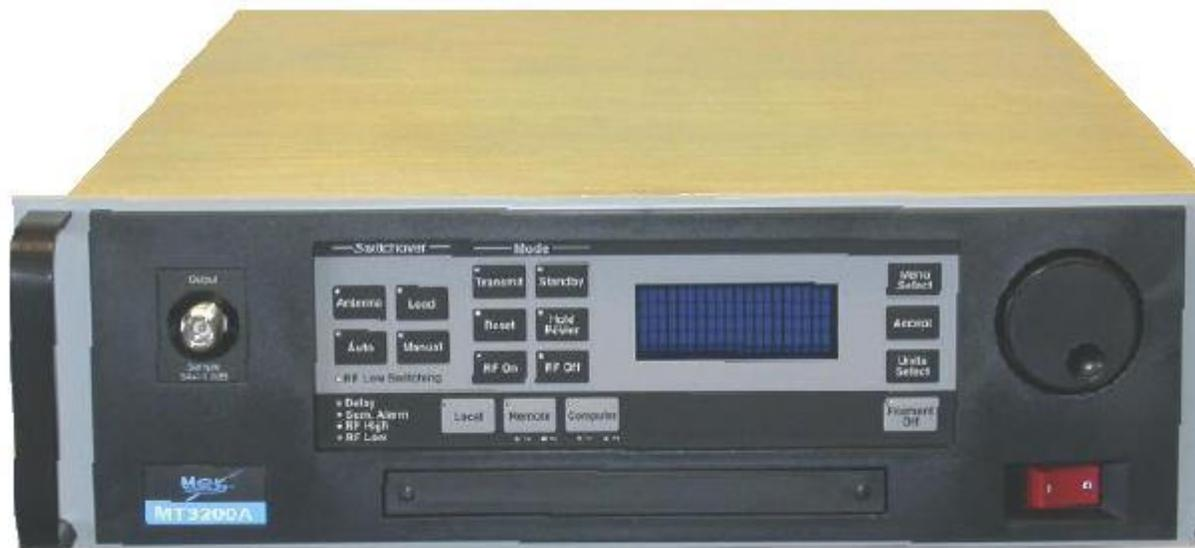
Rack mounted traveling wave tube equipment.
