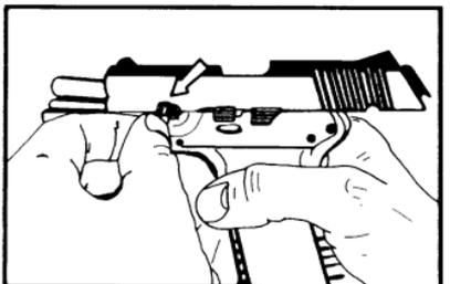
4. With left hand, pull SLIDE DISASSEMBLY LATCH or TAKE-DOWN PIN out of frame.
