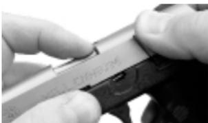
The slide may stick on the frame before going fully to the rear, or the barrel may ride with it to the rear. Begin again and press down with the finger onto that rear portion of the barrel accessible through the ejection port.
