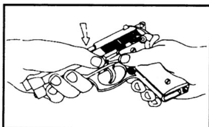
3. Pull forward the **SLIDE-BARREL** assembly.
