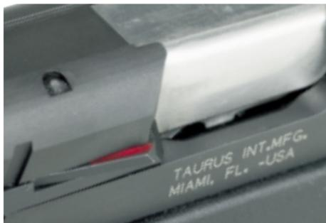
**chamber indicator.** To determine if chamber is loaded, make sure your finger is not on the trigger or inside the trigger guard and pull slide to rear and visually inspect the chamber. In any case, always inspect the chamber visually by pulling the slide back slowly and looking into the chamber while keeping your finger well clear of the trigger and trigger guard and keeping the muzzle pointed in a safe direction.
