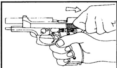
4. The pistol is now cocked and ready to fire by pulling the **TRIGGER**. After firing, the **SLIDE** will recoil from gas pressure and will eject the empty cartridge case and feed another cartridge into the chamber. The pistol will be ready to fire again. After the last round, the **SLIDE** will remain in the open position held by the **SLIDE CATCH**. In order to make it return to its rest position, press the **SLIDE CATCH** just above the **LEFT GRIP**.
