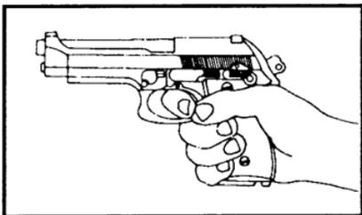
5. If you want to stop shooting before firing the last cartridge of a magazine, decock the firearm immediately by moving the safety downward and push the safety lever in the up (on) position.
