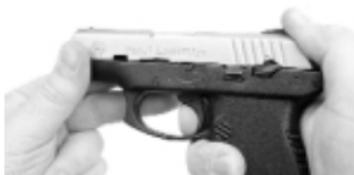
If the slide sticks on the frame, be sure the chamber is empty and firmly pull the trigger fully to the rear while pulling the slide forward off the frame.
