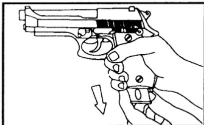
2. Hold the **MAGAZINE** with one of your hands and with the other one insert the cartridges one at a time, pressing them down and to the rear. Insert the **MAGAZINE** into the pistol until it is held by the **MAGAZINE CATCH**.
