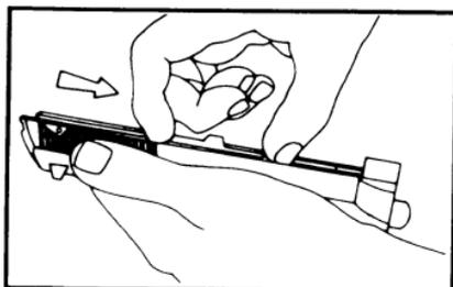
7. Remove BARREL from SLIDE by pulling to the rear and up.
