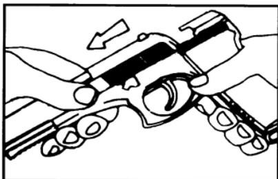
6. Carefully remove SLIDE SPRING and GUIDE from its position on the bottom of the BARREL. SPRING is under compression so it must be kept under control until removed.
